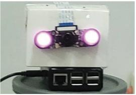
Figure 7: Physical IR Camera with Raspberry Pi
