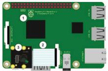
Figure 2: The schematic installation of CSI camera
