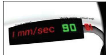
Fig. 7. The indicator for welding speed and angle on virtual welding torch.
