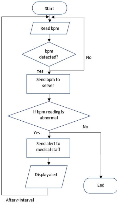
Fig. 3. The Flow Design of the System for Alert Module
