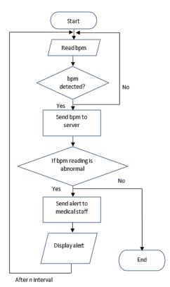
Fig. 3. The Flow Design of the System for Alert Module
