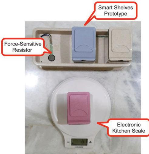
Fig. 6. Setup for the interoperability testing
