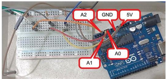
Fig. 5. Detailed view of the setup pins between the Arduino Uno and FSRs
