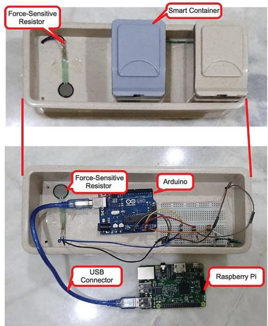
Fig. 4. Hardware implementation of the Smart Shelves prototype.
