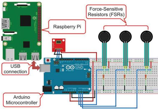
Fig. 3. Hardware schematic for the Arduino microcontroller and FSRs
