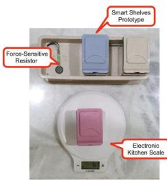
Fig. 6. Setup for the interoperability testing
