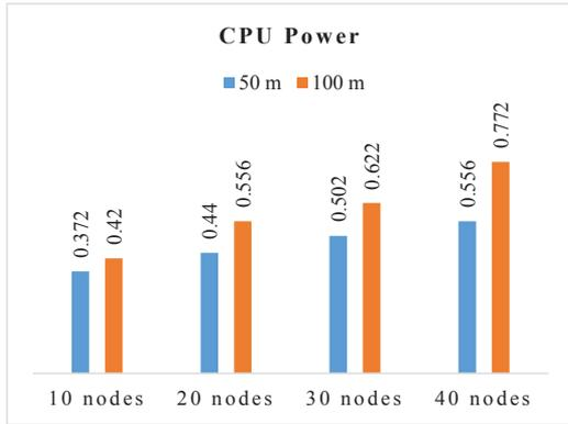
Fig.11. Comparison of CPU Power Between 50m and 100m TR
