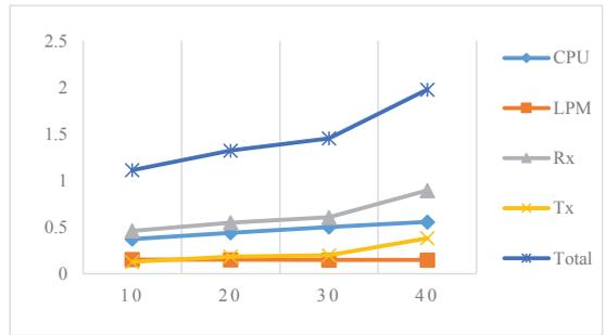
Fig. 9. Power Consumption Usage in 50 m Transmissions Range
