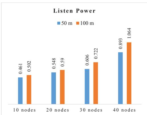
Fig.13. Comparison of Listen Power between 50 m TR and 100 m TR
